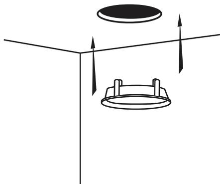
2. Remove the grille from the mounting flange by pressing it from behind. Insert the mounting flange into the hole. Loosen the flange clamping screws one turn (counter clockwise) to release the clamp. Next, tighten all four flange clamp screws evenly to secure the flange to the wall. It is best to tighten each screw with the same amount of force (torque). CAUTION: Do not over-tighten.
