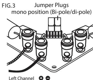
**Bi-pole/Di-pole FIG. 4 – 4 ohms:** Use this configuration for home theater surround applications. For bi-pole mode, connect as in the Mono/Stereo instructions (FIG.3): one speaker to each surround channel. For di-pole mode, connect speaker inputs the same as Mono/Stereo instructions (FIG.3), but reverse the + and - connections of the marked tweeter wires to put one of the tweeters out of phase.
