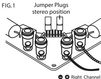
**Stereo Point Source FIG. 2 – 8 ohms:** Use this configuration to combine left and right channels for full fidelity sound from a single loud-speaker stereo source. Set jumper plugs in the stereo position. Connect right and left signal wires to the spring-loaded terminals on the rear of the speaker.
