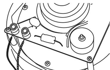
4. Carefully place the speaker in the flange. While exerting upward pressure, rotate the speaker until it fits snugly and the speaker surface is even with or slightly recessed into the surface of the flange. Twist the speaker counter-clockwise (left) to secure it in place. This will engage the QM SAFETY-LOC™ clamps on the back of the flange. Finish by tightening the four clamp screws on the speaker. CAUTION: Do not over-tighten.
