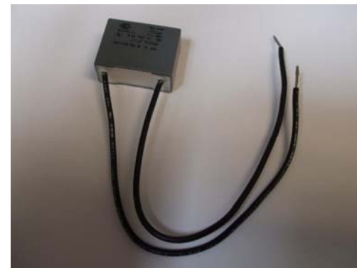
Shunt capacitor details: flying-lead, X1 rated, 310 VAC, 0.47 \mu F
