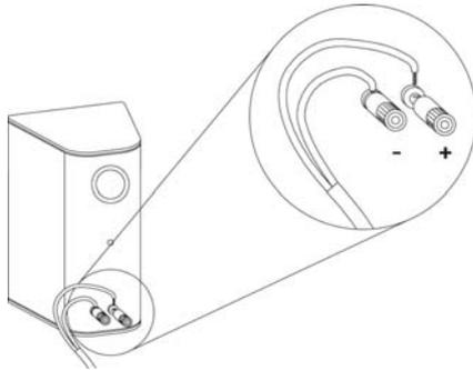
Pass the wires fully through the opening.
