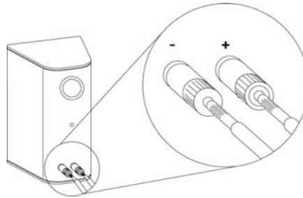
Fully insert the banana plugs up to the stop.
